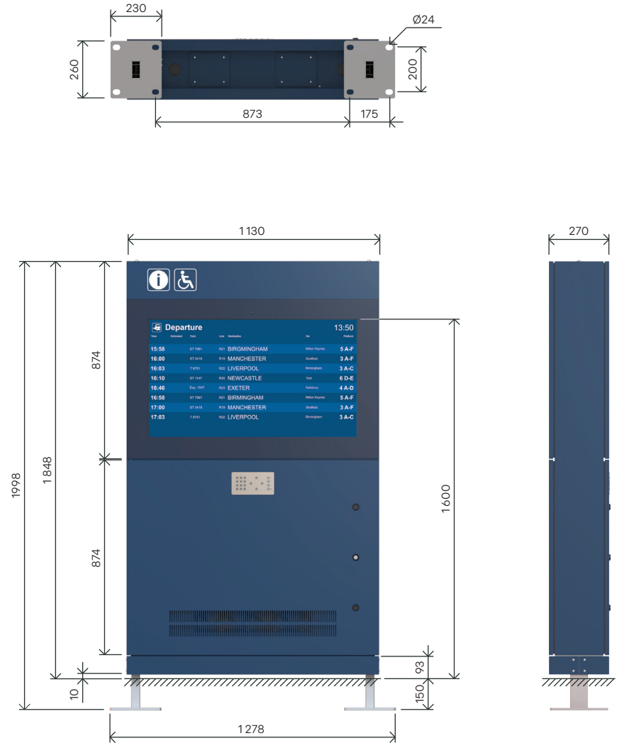
Double sided, mounting on prepared concrete foundation, frame and cover glass mask color RAL 5003
